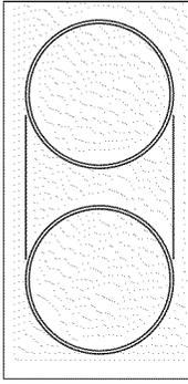
The Bridge element combines two individual heating elements into one long griddle zone. This configuration is ideal for griddles and large pans.
