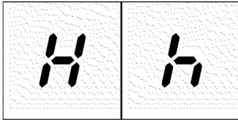
The cooktop has a hot surface indicator for each element. It shows you which elements are still hot. The hot surface indicator has two levels.
