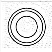
On this heating element you can turn the medium and large heating ribbons off. The heating element must be turned on.
