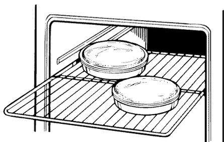
Hot air must circulate around the pans in the oven for even heat to reach all parts of the oven. This results in better baking.
