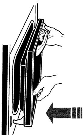
1. **Fit** hinge arms into slots in frame. **Push** in at lower corners to insure that hinge arms are fully engaged.
