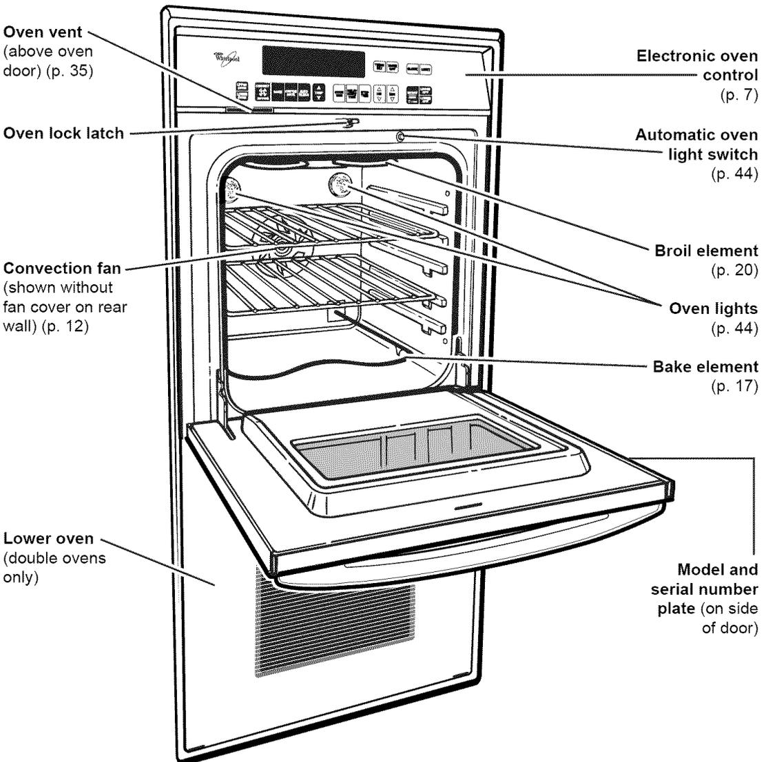
**NOTE:** Oven cooling fan remains on when oven is off until cavity temperature cools to 250°F.
