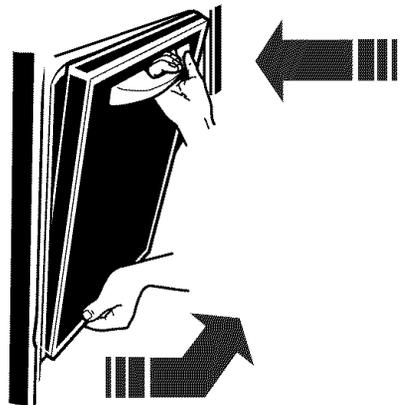
3. **Grasp** under handle and gently close door as far as it will shut. **Pull** door out at bottom to remove.
