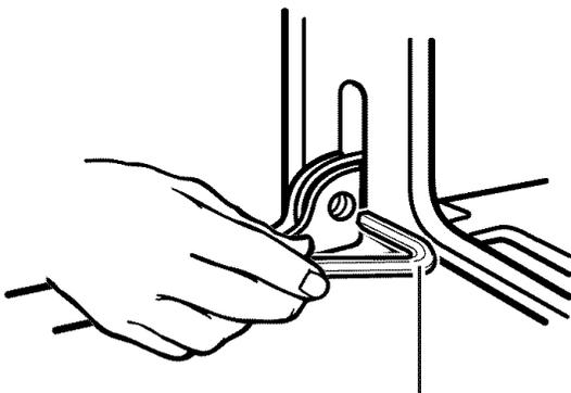
Insert small end of pin here
