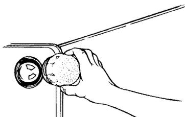
2. **Remove** the glass bulb cover in the back of the oven by screwing it out counter-clockwise.
