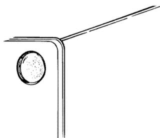
4. **Replace** the light bulb cover by screwing it in clockwise. The light bulb cover must be in place when using the oven. The cover protects the bulb from breaking and from high oven temperatures.
