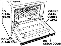
DO NOT clean, move or bend the fiberglass seal. Poor cleaning and poor baking will result.
