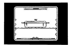
4. Put food in the oven. During baking, the elements will turn on and off to keep the oven temperature at the setting. The Oven HEATING Indicator Light will turn on and off with the elements.
