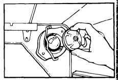
Remove the bulb cover in the back of the oven by pulling out and pushing the wire holder to the side.
