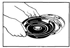
Line up openings in the reflector bowl and notches in the trim ring with the surface unit receptacle and the element hold down clip.
