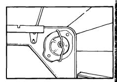
Replace the bulb cover and snap the wire holder in place. Plug in appliance or reconnect at the main power supply.
