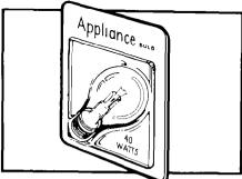
3. Remove the light bulb from its socket. Replace the bulb with a 40-watt appliance bulb.
