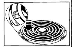
4. When terminal is pushed into the receptacle as far as it will go, push down the edge of the surface unit opposite the receptacle. The element hold down clip will keep the surface unit from moving around.
