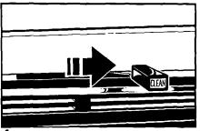
4. Move the Lock Lever to the right – the Clean position. The Oven HEATING and ON Indicator Lights will come on.
