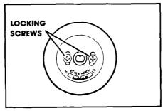
Loosen the locking screws inside the control knob. Note the position of the notches.
