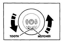
**3.** To lower the temperature, move the tooth a notch closer to LO. Each notch equals about 10°F (5°C).
