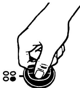
2. **Lift** the edge of the unit, opposite the receptacle, just enough to clear the element hold-down clip and the reflector bowl.
