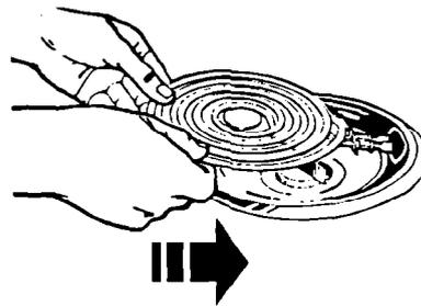
4. When the terminal is pushed into the receptacle as far as it will go, **push down** the edge of the surface unit opposite the receptacle. The element hold-down clip will keep the surface unit from moving around.
