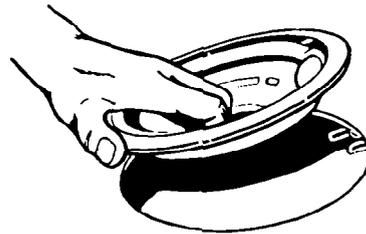
3. **Hold** the surface unit as level as possible with the terminal just started into the receptacle. **Push** the surface unit terminal into the receptacle.
