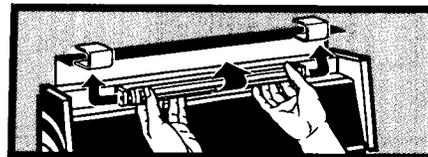
2. Remove lamp socket safety covers at each end of the fluorescent tube.
