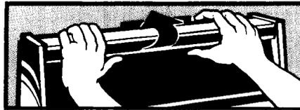
1. Flip up the console top by grasping it with both hands near each end and lifting the front edge up.
