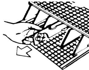
**To remove the basket**, slide it toward the top of the door—by the handle. Lift it off the holding buttons. Replace it in reverse order.
