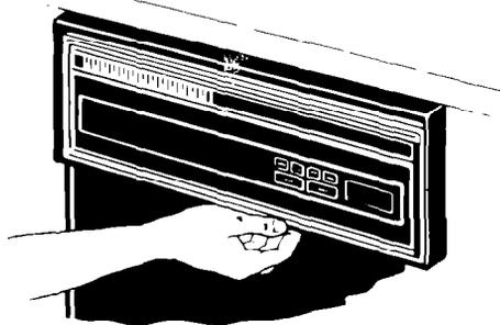
2. To stop the dishwasher, unlatch the door by pushing in the latch handle under the control panel. **Do not** open the door until the spray arms stop spinning. The DOOR OPEN indicator will flash and a tone will beep.
