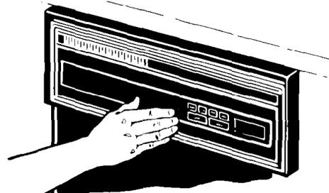
4. Close the door. **Do not latch it.** Wait 30 seconds for air in the dishwasher to warm up. This helps reduce the amount of moisture that can come from the vent when restarting the program.
