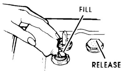
A rinse aid helps keep water from forming droplets and drying as spots. Keep the dispenser filled with a rinse aid such as Jet-Dry.<sup>®</sup> A small amount is released automatically during the final rinse of each cycle. Check the dispenser periodically to see if it needs refilling.
