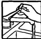
2. Hold a candy or meat thermometer in the running stream of water. If water temperature at the faucet is below 120°F (49°C), have a qualified person raise the water heater's thermostat setting.
