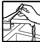
2. Hold a candy or meat thermometer in the running stream of water. If water temperature at the faucet is below 120°F (49°C), have a qualified person raise the water heater's thermostat setting.
