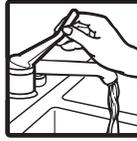
7. Press a Cycle pad. If desired, press one or more Option pads. See the “Setting the Controls” section. The dishwasher starts filling once you press a cycle pad unless you select the delay wash cycle. You may press Option pads as the machine is filling.
