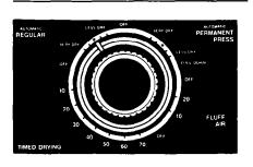
Select a cycle by turning the Cycle Control Knob either way. Stop when the indicator on the knob's outer ring points to the cycle and/or setting you want. See pages 6-7 for further cycle information.
