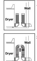
1. Clamp one elbow/vent section to the wall and one to the dryer
