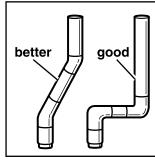
exhaust vent. Use the fewest number of elbows and turns. Allow room when using elbows or making turns. Bend vent gradually to avoid kinking.
