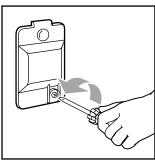
cover from the back wall of the dryer by removing the screw located in the lower right corner of the cover.
