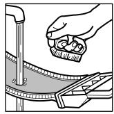
gent; scrub lint screen with the brush to remove residue buildup.
