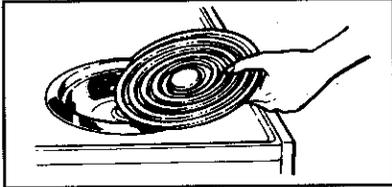
**To replace:** Insert the terminals on the element into the receptacle. Gently lift up on outer edge of element (opposite terminal-side of element) while inserting terminals into receptacle. Gently press down on outer edge of element until element sits level on drip bowl.
