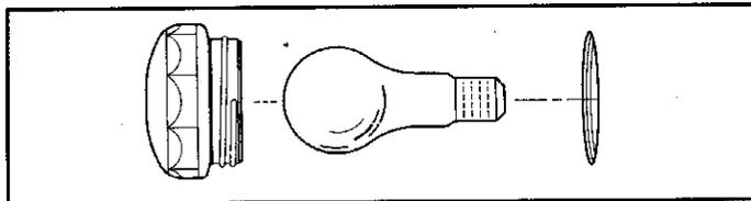
Replace with a 40 watt appliance bulb. Replace bulb cover and reconnect power to range. Reset the clock.
