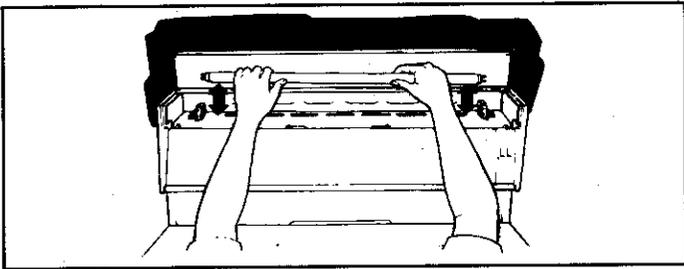
Remove fluorescent tube and replace with an 18 watt fluorescent tube. Snap top trim back into place and reconnect power to range. Reset the clock.
