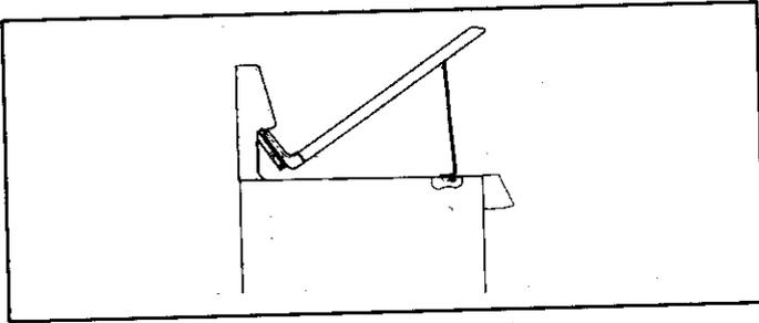
**To lower the top:** Hold the front edge of the cooktop and carefully push back on each support rod to release the notched support. Then gently lower the top into place. The support rods will slide into the range frame.
