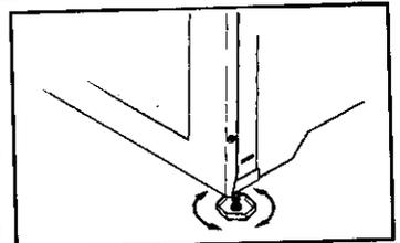
range should be secured to the floor by sliding a rear leveling leg into the anti-tip bracket supplied with the range.
