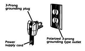
The compactor is for use on a 120-volt, 60 Hz, AC only 15 ampere fused and properly grounded circuit and is equipped with a grounding plug as shown above. For your personal safety, the compactor must be grounded. In the event of an electrical short circuit, grounding reduces the risk of electric shock by providing an escape wire for the electric current. This appliance is equipped with a polarized 3-prong grounding plug.
