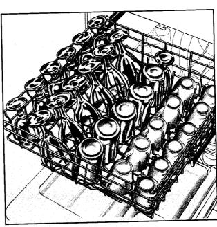
The upper rack may be removed if desired. Push inward on the front of the rack rail ends to unsnap. Remove rail ends and pull out rack.
