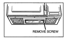
To replace cooktop light, first disconnect power at main fuse or circuit breaker panel or pull plug.
