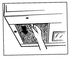
To remove grease filter, grasp the "finger hold" on the filter and slide to the rear.
