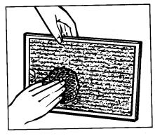
To clean grease filter, soak, then agitate filter in solution of hot water and detergent. Don't use ammonia or other alkali because they will darken metal. Light brushing can be used to remove embedded dirt. Rinse, shake and remove moisture before replacing. Filters should be cleaned at least once a month. Never operate your hood without the filter in place. In situations where flaming might occur on surfaces below hood, filter will retard entry of flames into the unit.
