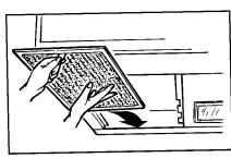
To replace grease filter, slide the filter in the frame slot on the back of the opening.
