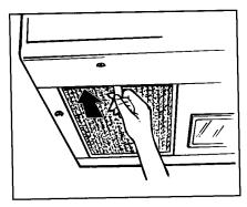
Pull filter upward and to the front to lock into place.
