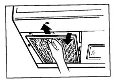
Then pull filter downward and to the front. The filter will drop out.
