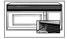
To replace your oven light, first disconnect power at main fuse or circuit breaker panel or pull plug. Remove the top grill by taking out the 2 screws that hold it in place.
