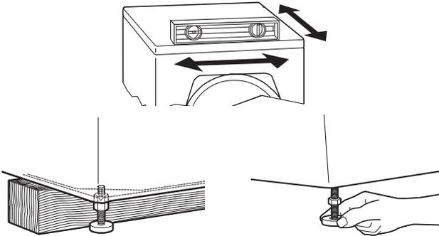
If the washer is against a wall, move the washer out slightly before tipping back. If the washer is not level, first prop the front with a wooden block and adjust the front feet height moving the hexagonal plastic part as necessary. Repeat to adjust back feet.
