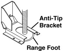
**Making sure the anti-tip bracket is installed:**
