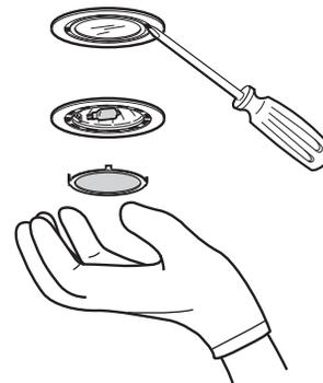
3. Remove the lamp and replace with a 12-volt, 20-watt maximum, halogen lamp made for a G-4 base.
