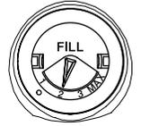
**NOTE:** For most water conditions, the factory setting of 2 will give good results. If you have hard water or notice rings or spots, try a higher setting. Turn the arrow adjuster inside the dispenser by either using your fingers or inserting a flat-blade screwdriver into the center of the arrow and turning.
