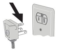
Power supply cord with 3-prong grounding plug
